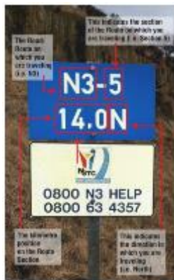
Figure 4-1: Typical kilometre marker with explanations
