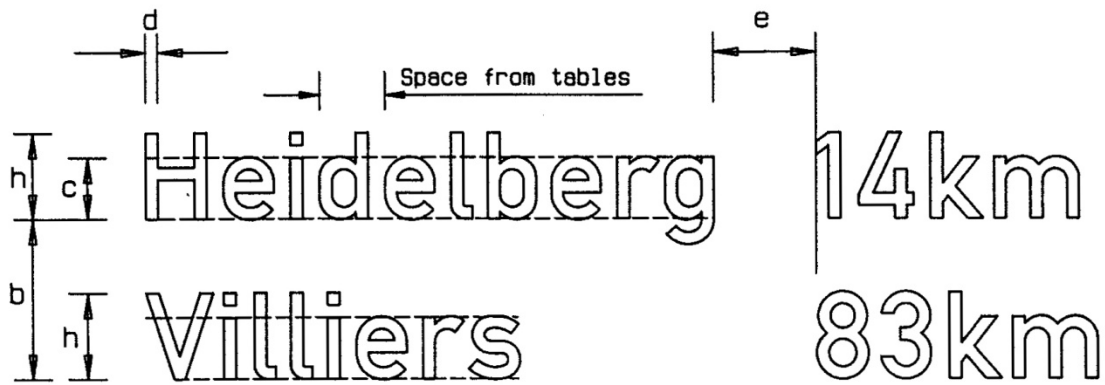
Fig 11.7 Letter and Word Dimensioning and Spacing
