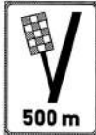
ARRESTOR BED ADVANCE EXIT SIGN
