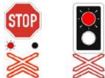
Flashing Red Disc (FRD) signal at railway crossings
