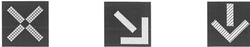
Detail 9.2.1 Overhead Light-emitting Lane Control VMS
