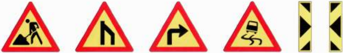
Detail 1.10.2 Temporary Warning Signs
