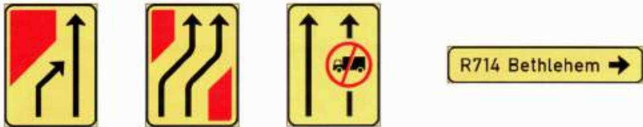
Detail 1.10.3 Temporary Guidance Signs
