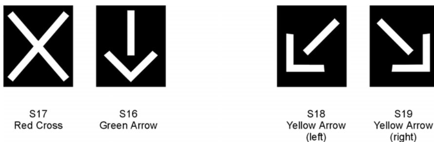
Figure 13.1: Standard lane direction control signals
