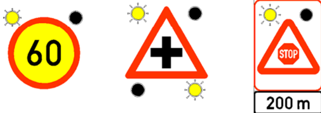
Flashing yellow warning signal SS3
