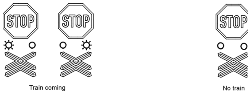
Figure 14.1: Flashing red disc light signals at railway crossings
